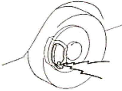
**The brake pad wear indicators on your disc brakes give a warning noise when the brake pads are worn to where replacement is required.**
