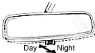
Pull the lever toward you to reduce the glare from the headlights of the vehicle behind you during night driving.
