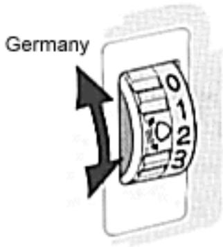
**To adjust the headlight beam level, turn the switch.**
