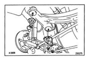
(b) Remove the 6 nuts and the left and right suspension member lower stopper.
