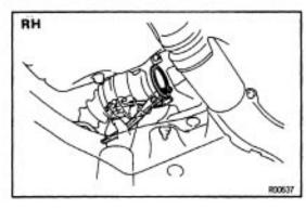
(b) Using pliers, remove the snap ring, and pull out the drive shaft.
