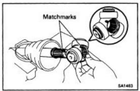
(c) Align the matchmarks placed before removal.
