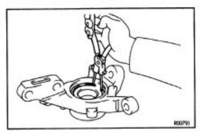
(b) Using snap ring pliers, install a new snap ring.
