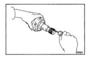
(b) Using a screwdriver, remove the snap ring.
