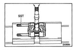
(b) Using SST and a press, press out the drive shaft side dust cover.
