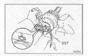
(h) Tighten SST so that the clamp is pinched.
