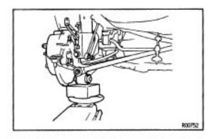
(b) Support the rear axle carrier with a jack.
