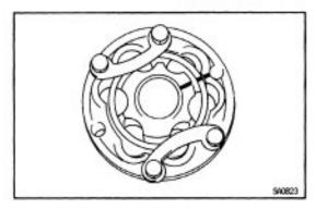
(e) Use bolts, nuts and washers to keep the inboard joint together.
