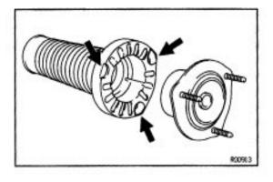
(b) Install the upper insulator to the upper support. HINT: Match the bolt of the upper support with the cut—off part of the insulator.
