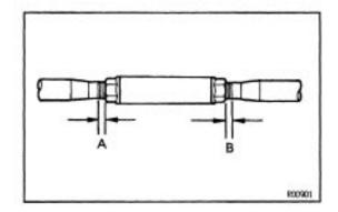
HINT: When assembling the No.2 lower suspension arm, try to make dimensions A and B shown in the illustration as close as possible.
