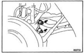
5. INSTALL LEFT AND RIGHT STABILIZER BAR LINKS Torque: 39 N·m (400 kgf·cm. 29 ft·lbf)
