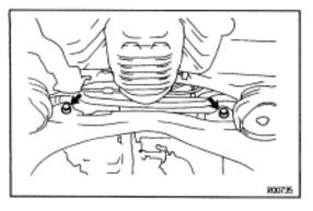
7. REMOVE STEERING GEAR BOX MOUNTING BOLTS AND NUTS
