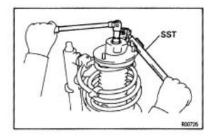
(c) Using SST to hold the upper support remove the nut. SST 09729–22031
