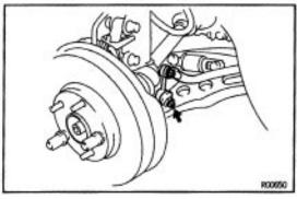
6. CONNECT STABILIZER BAR LINK TO LOWER ARM Torque: 39 N·m (400 kgf·cm, 29 ft·lbf)
