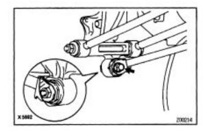
(b) Remove the bolt and nut and disconnect the strut rod from the rear axle carrier.
