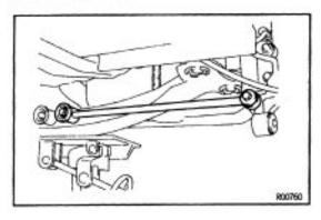
(d) Remove the No. 1 lower suspension arm with the 2 bolts and the washer.
