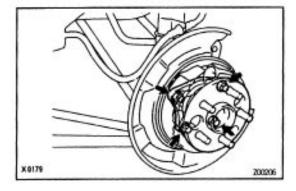
(b) Install the rear axle hub with the 4 bolts.
