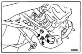
(b) Connect the lower ball joint to the lower arm and tighten the bolt and nuts.
