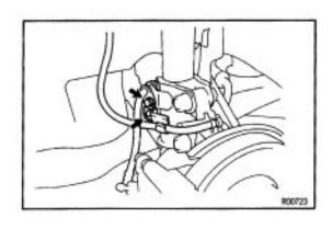
7. INSTALL BRAKE HOSE AND ABS SPEED SENSOR WIRE (W/ ABS) TO SHOCK ABSORBER
