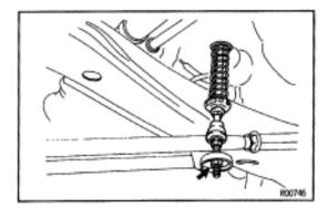
4. REMOVE ABS SPEED SENSOR WIRE (w/ ABS) AND BRAKE HOSE FROM SHOCK ABSORBER
