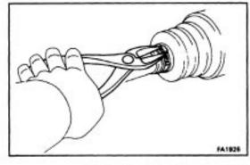
(b) Using side cutters, cut the small boot clamps and remove them.
