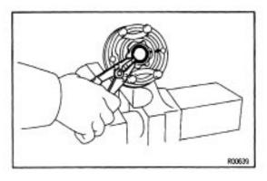
(b) Using a snap ring expander remove the snap ring.
