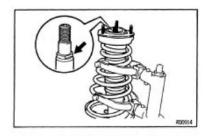
(c) Install the upper support to the piston rod.
