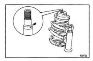
(b) Install the upper support to the piston rod.
