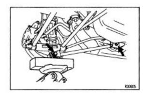
(h) Torque the strut rod set bolts.
