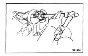
(d) Using a brass bar and hammer, tap in the tripod joint to the drive shaft.
