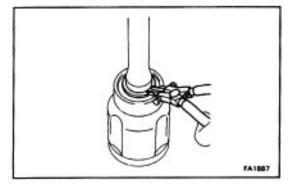
(c) Using a snap ring expander, install a new snap ring.
