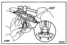
(b) Using SST, remove the inner race (outside) from the axle shaft.
