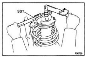
(c) Using SST to hold the upper support, install a new nut. SST 09729–20031
