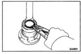
(c) Using snap ring pliers, remove the snap ring.
