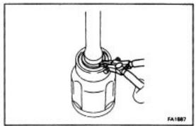
(b) Using a snap ring expander, remove the snap ring.
