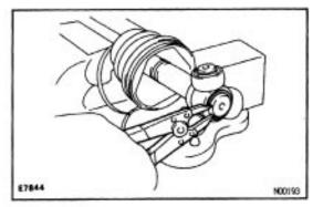
(e) Using a snap ring expander, install a new snap ring.
