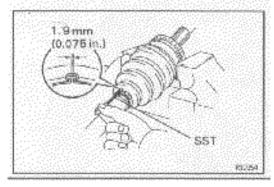
(i) Using SST, adjust the clearance of the clamp. SST 09240 – 00020
