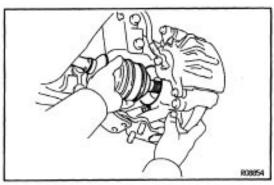
2. INSTALL DRIVE SHAFT TO AXLE HUB
