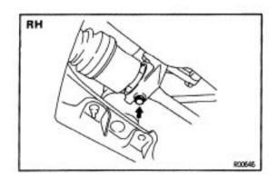
(d) Install a new bearing lock bolt and tighten it.
