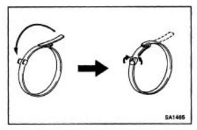
(c) Using a screwdriver, bend the band and lock it as shown in the illustration.
