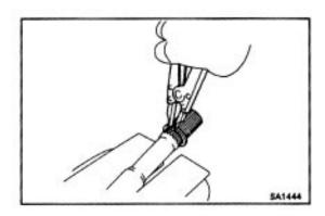
(e) Using a snap ring expander, remove the snap ring.
