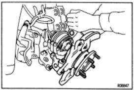
(b) Remove the steering knuckle with axle hub.
