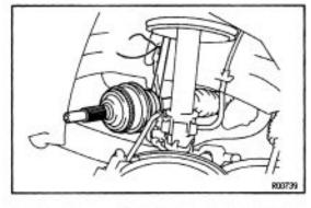
(b) Hang up the drive shaft using wire, etc.
