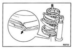
(b) Install the coil spring to the shock absorber. HINT: Fit the lower end of the coil spring into the gap of the lower seat.
