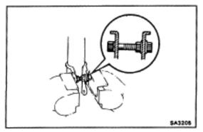
(b) Install a bolt and 2 nuts to the bracket at the lower portion of the shock absorber and secure it in a vise.
