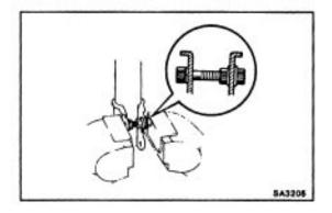
(c) Install a bolt and 2 nuts to the bracket at the lower portion of the shock absorber and secure it in a visa.
