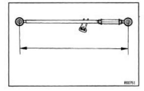
(c) Adjust the No.2 lower suspension arm length by turn—ing the adjusting tube.
