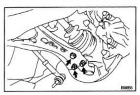
**3. CONNECT LOWER ARM TO LOWER BALL JOINT** Install the bolt and 2 nuts.
