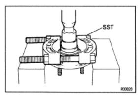
(b) Using SST and a press, remove the inner race (outside) from the axle hub.
