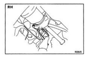
(b) Using pliers, remove the snap ring, and pull out the drive shaft.
