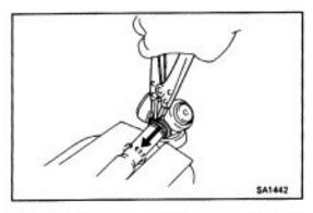
(b) Using a snap ring expander, temporarily, slide the snap ring toward the outboard joint side.
