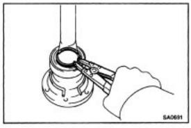
(c) Using a snap ring expander, install a new snap ring.
