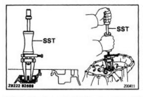
(b) Using SST, pull out the bearing. SST 09308–00010
