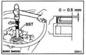
(b) Using SST, drive in a new oil seal.
