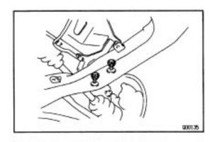
(c) Install and torque the 2 nuts.
