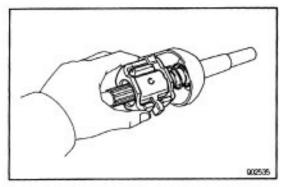
(b) Remove the shift interlock plate, shift inner lever No.1 and select spring seat.
