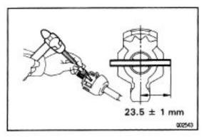
(c) Using a pin punch and hammer, drive in the slotted spring pin.
