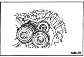
(b) Install the reverse idler gear and shaft as shown.
