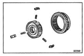
6. REMOVE NO.1 HUB SLEEVE, SHIFTING KEYS AND SPRINGS FROM NO.1 CLUTCH HUB
