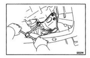
(c) Remove the 3 bolts and engine left mounting.
