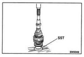
(d) Using SST and a press, install the rear ball bearing. SST 09608–12010 (09608–00070)
