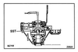
(g) Using SST and torque meter, measure the preload. SST 09564–32011
