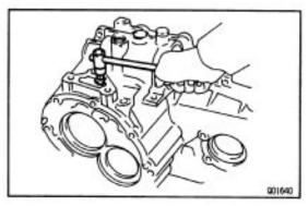
(e) Apply sealant to the plug threads.
