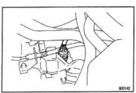
11. DISCONNECT VEHICLE SPEED SENSOR CONNECTOR
