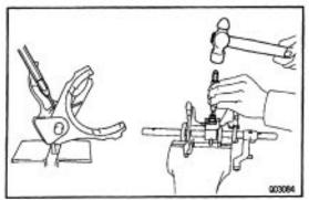
(c) Using a pin punch and hammer, drive out the slotted spring pin from the No. 1 fork shaft as shown in the illustration.
