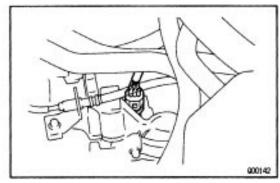
16. CONNECT VEHICLE SPEED SENSOR CONNECTOR
