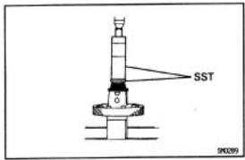
(c) Using SST and a press, install the side bearing to the transaxle case side.
