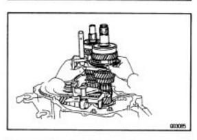
5. INSTALL NO.1 SHIFT FORK SHAFT, NO.1 SHIFT HEAD, NO.1, NO.2 SHIFT FORKS, REVERSE SHIFT FORK WITH INTERLOCK PIN, INPUT AND OUTPUT SHAFT ASSEMBLY
