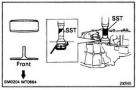
(c) Using SST, press in a new bearing. SST 09310–35010
