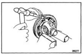
(g) Using a pin punch and hammer, stake the lock plates. HINT: Stake one claw flush with the flat surface of the bolt. For the claw contacting the protruding portion of the bolt, stake only the tightened side.
