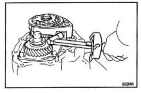
(b) Install and torque the set bolt.
