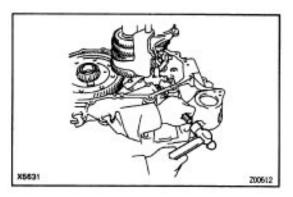
(b) Using a pin punch and hammer, drive in the slotted spring pin.
