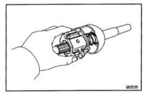
(b) Install the shift inner lever No. 1 with the shift interlock plate.
