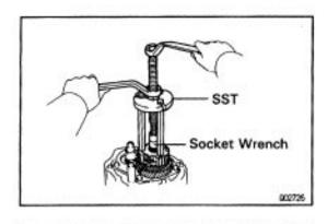
(b) Using SST, remove the No–3 clutch hub with syn-chronizer ring.
