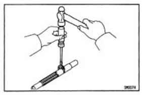
3. INSTALL E-RING TO SHIFT AND SELECT LEVER SHAFT
