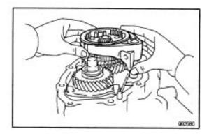
(b) Remove the No.3 hub sleeve and No.3 shift fork.
