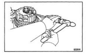
(c) Using a screwdriver and hammer, tap in the snap ring.
