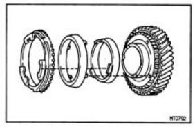
(c) Place the synchronizer rings on the 2nd gear.
