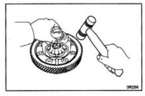
(d) Using a copper hammer, tap on the ring gear to remove it from the case.
