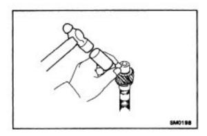
(c) Using a screwdriver and hammer, drive out the thrust washer.
