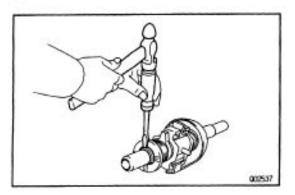
(b) Using a screwdriver and hammer, tap in the E-ring.
