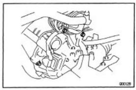
10. REMOVE TRANSAXLE MOUNTING THREE BOLTS OF TRANSAXLE CASE UPPER SIDE
