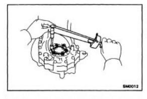
(c) Apply sealant to the bolt threads.
