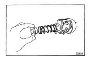
(b) Remove the reverse restrict pin holder, spring and shift inner lever No.2.
