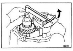
(b) Install and torque the new lock nut.
