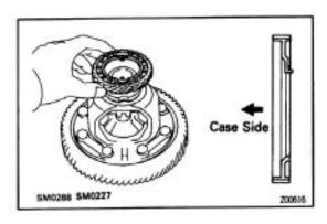
(b) Install the speed sensor drive gear to the transaxle case side.
