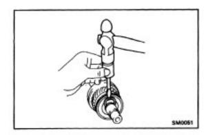
(b) Using a screwdriver and hammer, tap in the snap ring.
