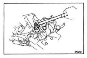
28. INSTALL BACK-UP LIGHT SWITCH Torque: 44 N-m 1450 kgf-cm, 33 ft.-lbf
