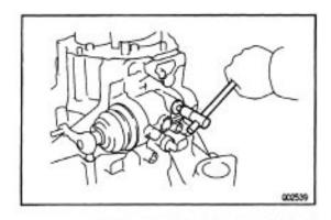
(b) Using a hexagon wrench, remove the plug.
