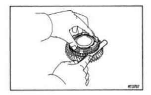
(c) Measure the clearance between the synchronizer ring back and gear spline end.
