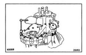
(c) Install and torque the 17 bolts.
