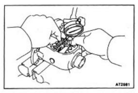
(d) Using a pin punch and hammer, drive in the straight pin through the case and hole in the pinion shaft.
