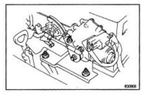
4. REMOVE CLUTCH RELEASE CYLINDER AND TUBE CLAMP
