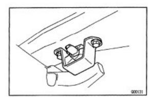
(c) Remove 2 bolts and exhaust pipe.
