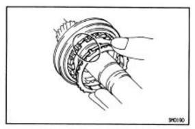
(c) Place the synchronizer ring on the gear. HINT: Align the ring slots with the shifting keys, and the ring projections with the hub slots.
