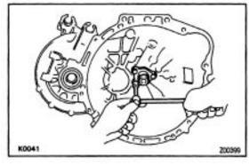
2. REMOVE RELEASE BEARING RETAINER
